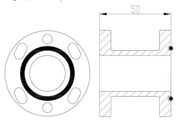
Flange 3/4/6 holes - Spacer 22mm
