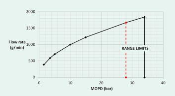
Flow rate with differential pressure 3,5 bar: 590 g/min. Oil: Reniso SP46 at +20 °C
